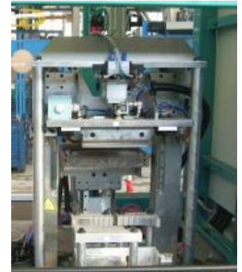
Hot Plate Welding
