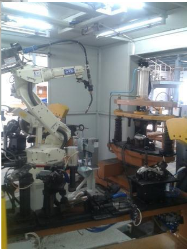
Robotic Welding Cell – Exmani + Catcon
